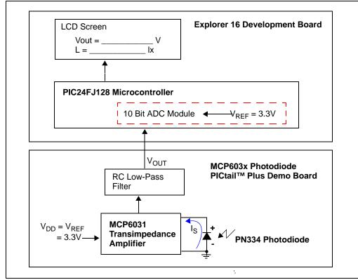
**FIGURE 1-2:** MCP6031 Photodiode PICtail<sup>™</sup> Plus Demo Board Function Block Diagram.
