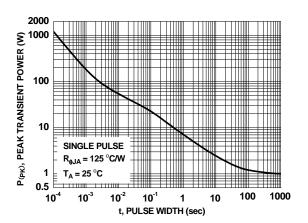
Figure 12. Single Pulse Maximum Power Dissipation
