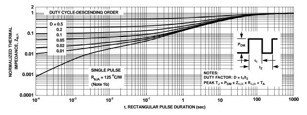
Figure 13. Junction-to-Ambient Transient Thermal Response Curve
