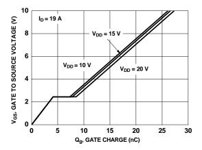
Figure 7. Gate Charge Characteristics
