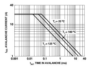
Figure 9. Unclamped Inductive Switching Capability
