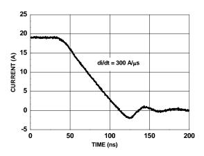
Figure 14. FDMS0310AS SyncFET<sup>TM</sup> body diode reverse recovery characteristic
