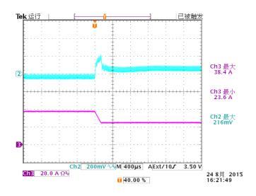
Figure 12: Output voltage response to step-change in load current (75%-50% of Io, max; di/dt = 0.1A/ $\mu$ s, Vin=54V). Load cap: 10 $\mu$ F, tantalum capacitor and 1 $\mu$ F ceramic capacitor. Top Trace: Vout (200mV/div, 400us/div); Bottom Trace: Io (20A/div, 400us/div). Scope measurement should be made using a BNC cable (length shorter than 20 inches). Position the load between 51 mm to 76 mm (2 inches to 3 inches) from the module.
