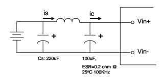
Figure 14: Test set-up diagram showing measurement points for Input Terminal Ripple Current and Input Reflected Ripple Current.
