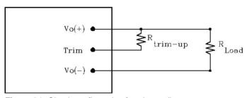
**Figure 21:** Circuit configuration for trim-up (increase output voltage)
