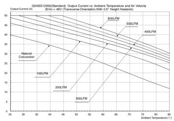
**Figure 26:** Output power vs. ambient temperature and air velocity @Vin=48V(Transverse Orientation, airflow from Vin- to Vin+, with 0.5" height heat sink)
