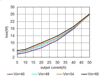
**Figure 2**: Power dissipation vs. load current for minimum, nominal, and maximum input voltage at 25°C(For module without current sharing)
