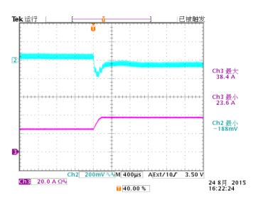
Figure 13: Output voltage response to step-change in load current (50%-75% of Io, max; di/dt = 0.1A/μs, Vin=54V). Load cap: 10μF, tantalum capacitor and 1μF ceramic capacitor. Top Trace: Vout (200mV/div, 400us/div); Bottom Trace: Io (20A/div, 400us/div). Scope measurement should be made using a BNC cable (length shorter than 20 inches). Position the load between 51 mm to 76 mm (2 inches to 3 inches) from the module.
