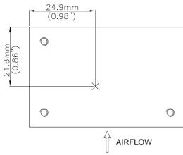
**Figure 23:** \* Hot spot 1 temperature measured point. the allowed maximum hot spot temperature is defined at 102  $\mathcal C$
