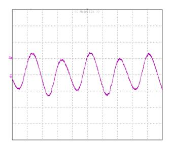
**Figure 15:** Input Terminal Ripple Current, i<sub>c</sub>, at full rated output current and nominal input voltage with 12μH source impedance and 100μF electrolytic capacitor (500 mA/div, 2us/div).
