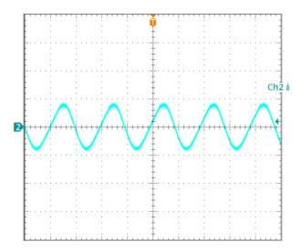
Figure 18: Output voltage ripple at nominal input voltage and rated load current (100 mV/div, 2us/div)
