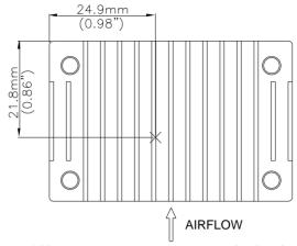
**Figure 24:** \* Hot spot 2 temperature measured point. the allowed maximum hot spot temperature is defined at 90  $^{\circ}$ C
