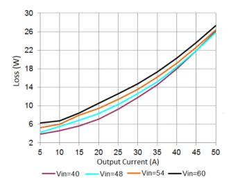
**Figure 4**: Power dissipation vs. load current for minimum, nominal, and maximum input voltage at 25°C(For module with current sharing)
