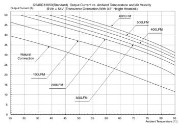
Figure 28: Output power vs. ambient temperature and air velocity @Vin=54V(Transverse Orientation, airflow from Vin- to Vin+, with 0.5" height heat sink)
