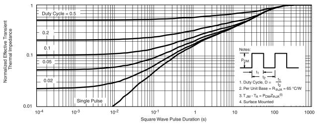
Normalized Thermal Transient Impedance, Junction-to-Ambient
