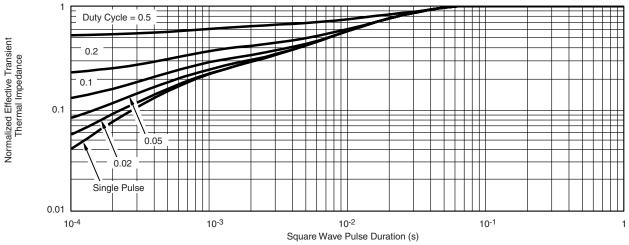
Normalized Thermal Transient Impedance, Junction-to-Case
