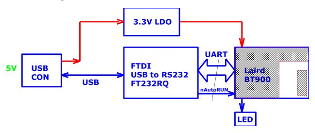
Figure 1: BT900-US block diagram
