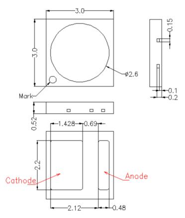
Note: The mark (dot) on top of the LED indicates the cathode for products manufactured in October 2016 and later. Products manufactured before October 2016 have the mark (dot) on the anode side.
