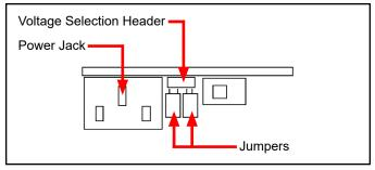
Figure 3. 110V jumper setting
