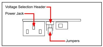
Figure 4. 220V jumper setting
