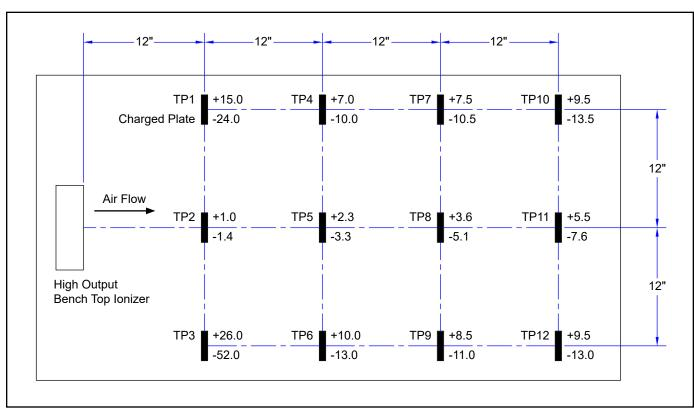
Figure 5. Neutralization (Discharge) Times at 120VAC / 220VAC, 60Hz input
