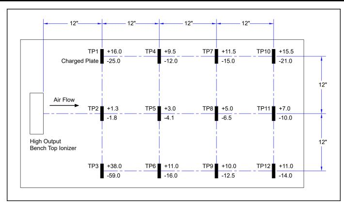
Figure 6. Neutralization (Discharge) Times at 100VAC, 50Hz input
