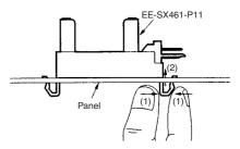
Pressed mounting holes are ideal for mounting the
