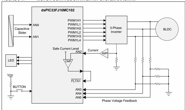
The application side of the starter kit is centered on the dsPIC33FJ16MC102 DSC, which requires very little additional hardware to perform its tasks. The Motor Control Starter Kit is preprogrammed with an application featuring integrated motor control and mTouch functionality. The motor control application algorithm is based on the application note AN1160 "Sensorless BLDC Control with Back-EMF Filtering Using a Majority Function".
