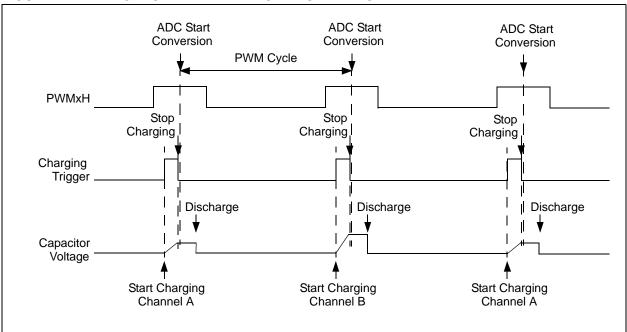
The CTMU module uses a trigger to start and stop charging of the slider's capacitors. The trigger is configured in such a way that the ADC starts conversion a few nanoseconds after the capacitor has stopped charging. This ensures that no PWM switching occurs while sampling the voltage on the capacitor.
